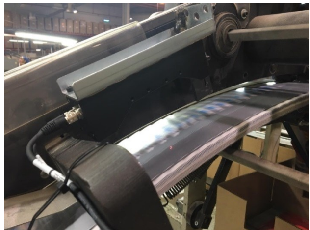
RED-110-L deployed in a laser copy counter application
